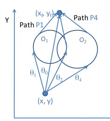
Shortest path: straight line to target
