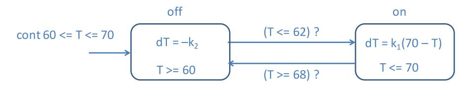
State machine with two modes: on and off
