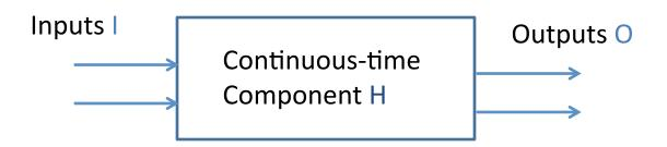
With a fixed initial state, a continuous-time component H maps input signals I(t) to output signals O(t)
