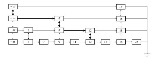
Figure 3: Example of a deterministic skip list where the higher level is created by picking alternate elements from the lower level. The bold arrows show the path taken by a search query for element 14 (since 14 is not in the list, we return the closest smaller element 12). The  $-\infty$  elements are added at the beginning for convenience and to give the search algorithm a concrete starting point irrespective of the changes in the data structure.
