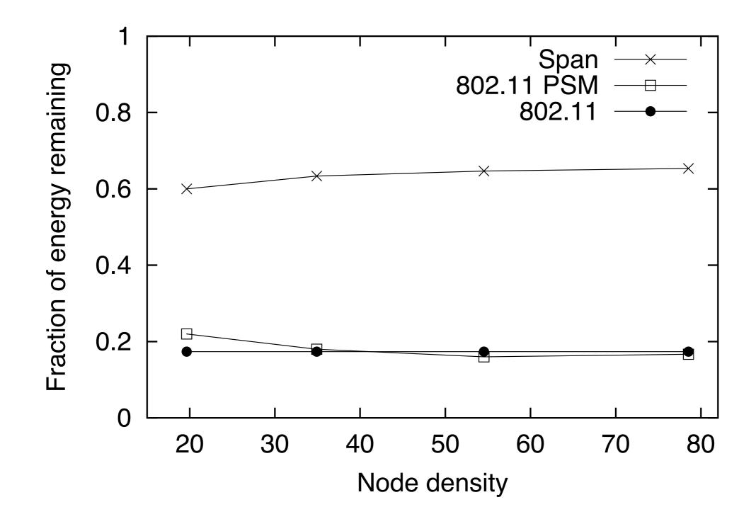
Figure 8: Fraction of energy remaining after 300 seconds of simulation. Span provides significant amount of savings over 802.11 PSM and 802.11.
