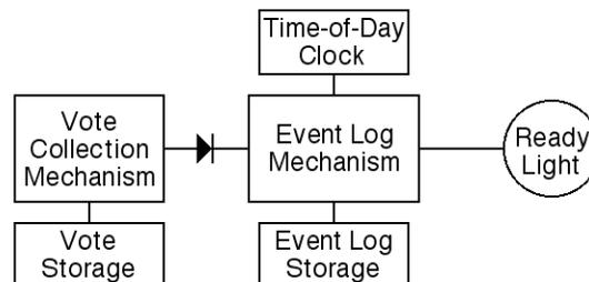
Figure 4: A data diode within a voting machine
