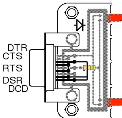
In the alternative cable suggested for connecting the source computer system to the RS-232 Data Diode, these “loopback” connections are wired inside the cable.
