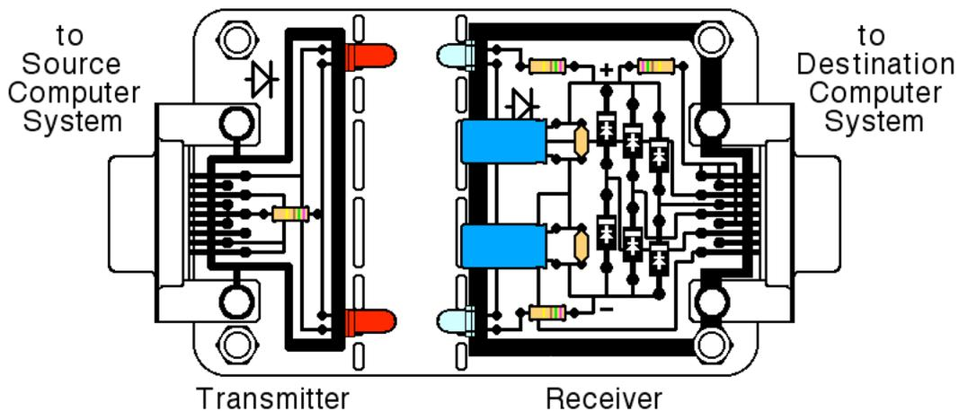
The transmitter converts electrical signals from the source computer system to optical form, using a pair of red LEDs. The receiver uses a pair of phototransistors to convert the optical data back to electrical form. The top LED/phototransistor pair transmits positive signals, while the bottom pair transmits negative signals.
