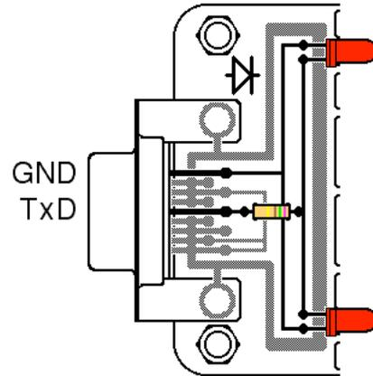
**The shielding loop** is a conductor that is tied to the shell of the cable connector, and through the cable connector to the shield of the cable.
