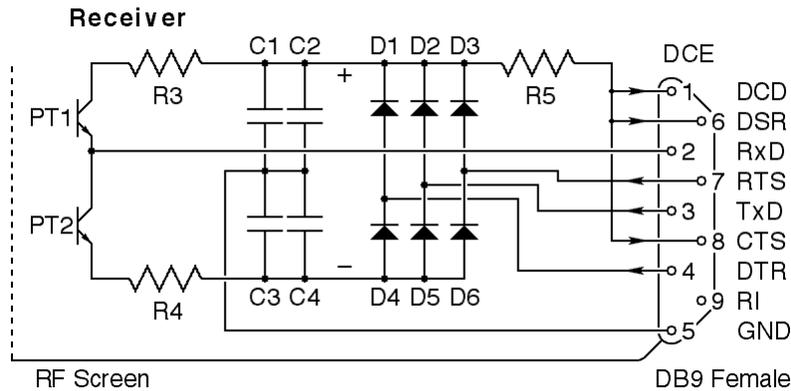
PT1 and PT2 – NPN phototransistors; PNA1801LS, able to handle a maximum forward current of 20 milliamps and a forward voltage of 15 volts or more, with a collector current of at least 3mA at 500 Lux, peak sensitivity near 800nm, and a 4 $\mu$ s response time. Redesign with a transistor amplifier on each phototransistor should increase the data rate.
