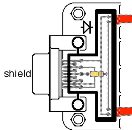
**The loopback connections** only matter if the cable to the source computer system includes connections for the DTR, CTS, RTS, DSR and DCD signals.
