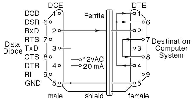
**The alternative destination cable using DC power** is identical to the AC alternative, except for the power provisions.
