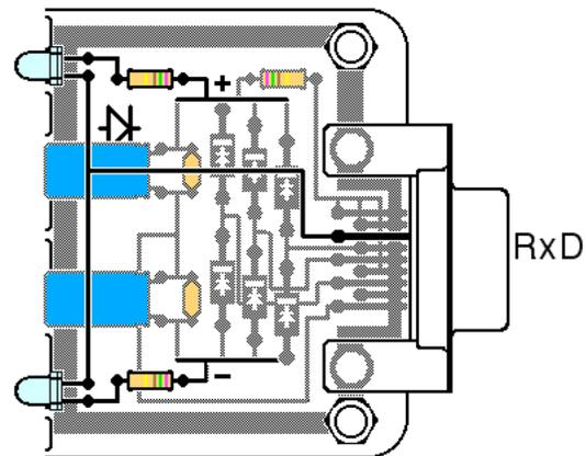
**The shielding loop** operates identically to that in the transmitter, except that it is also in electrical contact with the screws attaching the RS-232 Data Diode to its case.
