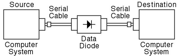
Each computer system sees the RS-232 Data Diode as a piece of data communications equipment (DCE). The serial ports of most computer systems conform to the standards for data terminal equipment (DTE). Therefore, the RS-232 Data Diode usually uses a pair of DCE to DTE cables. The most common cable, used with TIA 457 (IBM PC compatible) 9-pin serial ports, is wired as follows:
