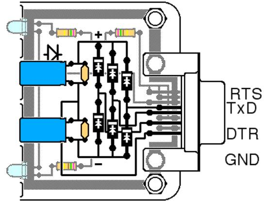
**The receiver circuit** uses the power supply to deliver a signal to RxD (pin 2).
