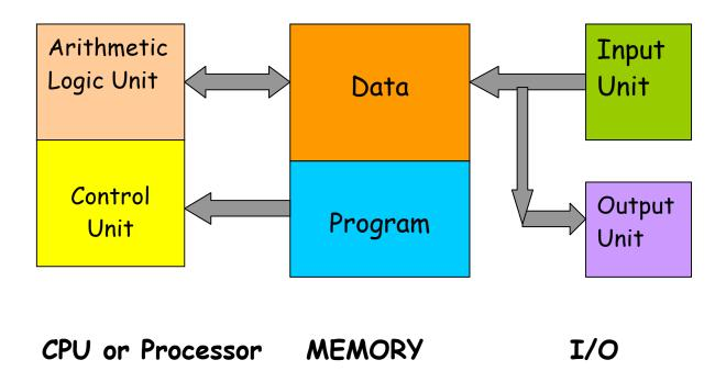
There are different ways of designing the "boxes" or the functional units. At the upper level, we care only about the functionality and not so much about their internal construction.
