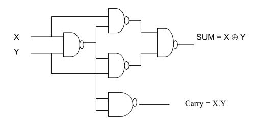
There are other circuits that take 5 gates to implement XOR, and can be derived from the definition of XOR  $x \oplus y = x.y' + x'.y$ . First implement it using AND OR NOT gates, and then substitute each gate with its NAND equivalent (we have already done this exercise when we studied why NAND gates are universal gates. See Section 3.3.2 pp 103-104).
