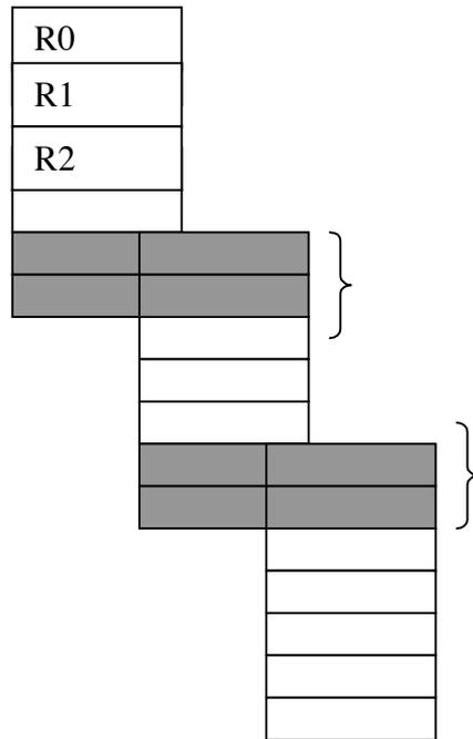
The called procedures use a different set of physical registers. Thus the architectural registers R0-R31 are essentially renamed. The overlapped sections simplify parameter passing.
